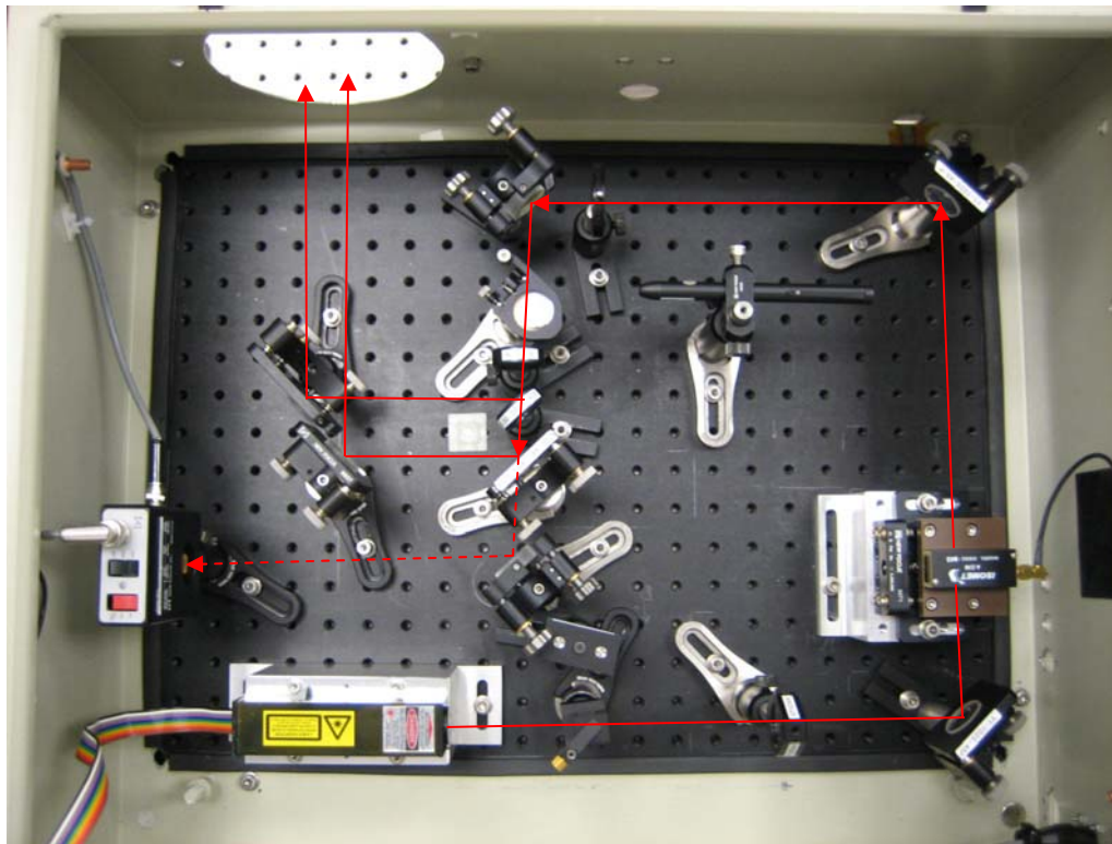
Figure 3 Bird's-eye view of proposed layout upgrade. The two-beam output configuration is shown. The horizontally-polarized laser output passes through a polarizing beamsplitter cube before being focused into the AOM. The first order diffracted beam is then focused by a single spherical lens on the way to a 50%
