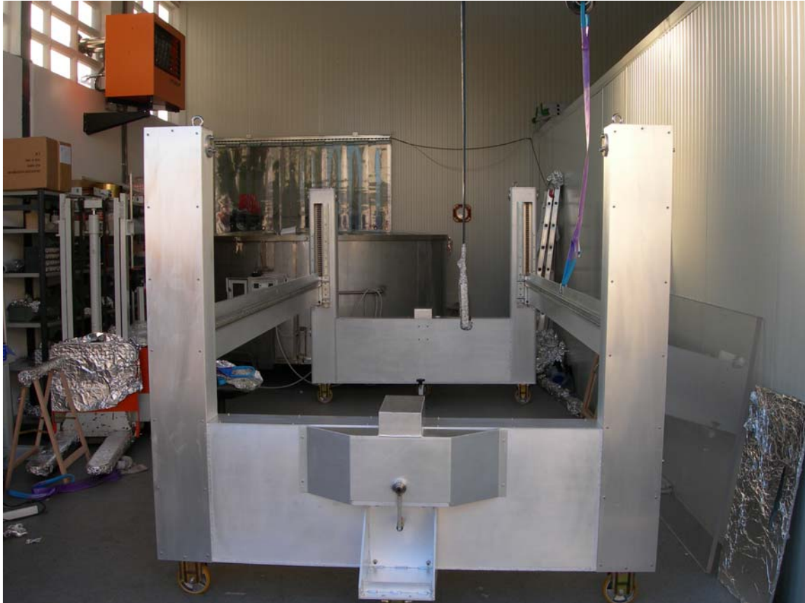
Figure A3-6. Elevator/insertion structure in the G&M grey room, before packing and shipping. The rails are lifted by turning the cranks, one of which is visible in the foreground.
