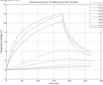
Note that multiple time scales likely apply and a steady-state was not achieved in this ~3hr heating test. The locations of the thermistors are shown here:
