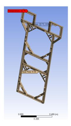
The surface total hemispherical emissivity of the aluminum structure is assumed to be 0.05, which is appropriate for 6061 Al alloy polished and degreased1. If the aluminum is 120 size, grit blasted then the emissivity is 0.40. However, this treatment may not be compatible with ultra-high vacuum (UHV) practice. It may be possible to increase the surface emissivity for temperature control in a UHV compatible manner, but this was not assumed in the analysis.
