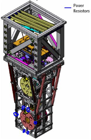
With 20W of total power dissipation equally split in these 6 resistors, the temperature response is:
