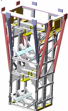
The details of the planar truss is simplified and then meshed for thermal analysis with Ansys:
