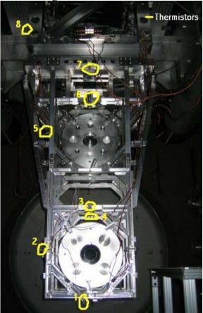
Due to the considerable thermal mass of the seismic isolation table, and to some extent the upper structure of the quad, one can approximate the interface of the lower structure and the upper structure as a constant temperature boundary condition in the early time history of the response to a ring heater in the vicinity of the test mass. The lower structure basically consists of 4 vertical aluminum plates which are machined into monolithic, planar truss structures.
