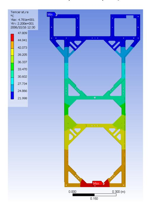
Transient analysis shows ~10C rise at the lower thermistors after 1 hr (3600 sec), as compared to ~8.5 C from experimental results.
