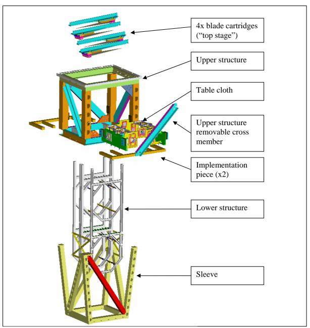
Note: The exploded view is for reference only and is not of the latest CAD model.
