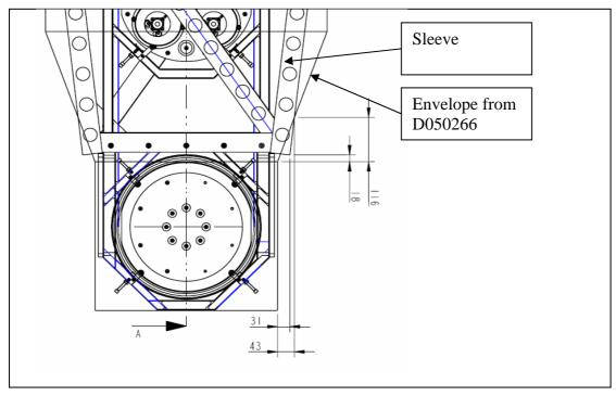
The figure above shows the infringement when looking along the beam and is dimensioned on one side, the infringement in the side view is very much smaller with no more than 5mm protruding outside the envelope.
