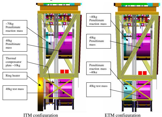
One of the most noticeable features of the noise prototype design is that the test and reaction chain thickness are different. This decision was made quite early in the noise prototype design process as the most robust way to make a stiff structure that fell within the envelope given by D050266. The complete argument is available in T050077, but could be condensed as follows:
