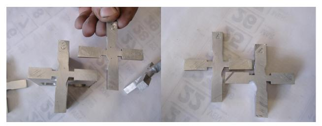
These welds present small cavities, that appear to be short (do not extend for the full or most of the length of the weld as in some of the previous tests) and while a large fraction of the landings between the tapered plates and the cross plate are molten, not everywhere the gap is closed.
