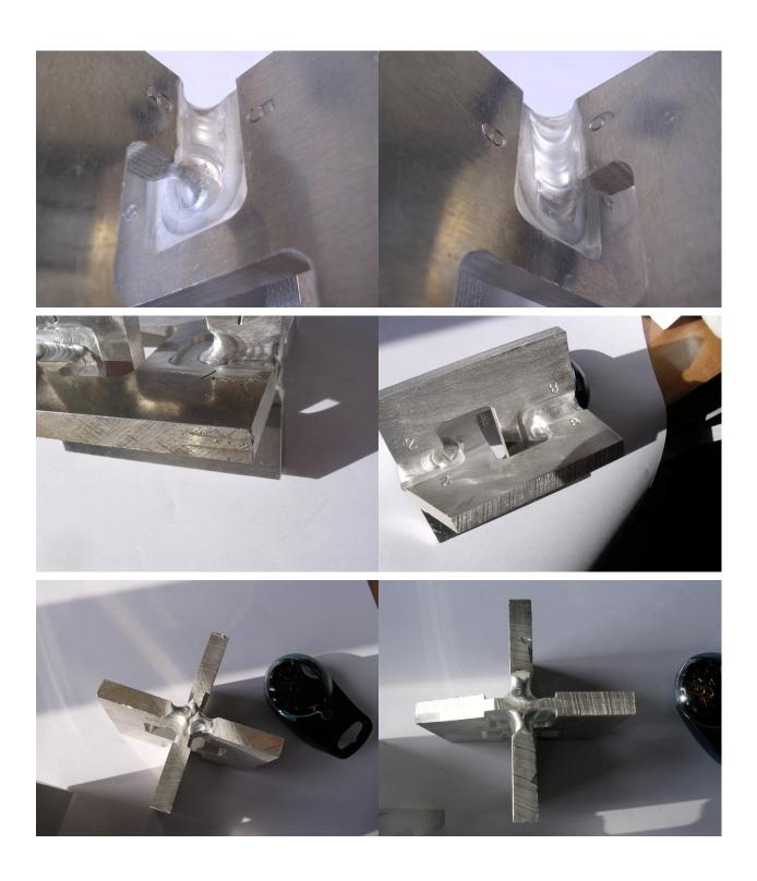
View from the inside point of view of the 8 welds of the **second** test sample and edge view of the two sides of the crosses.
