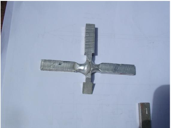
We conclude that with the machined geometry, the cross welds satisfy the LIGO requirements. Welds with an opening larger than  $90^{\circ}$  are satisfactory and produce the desiredfull penetration welds.
