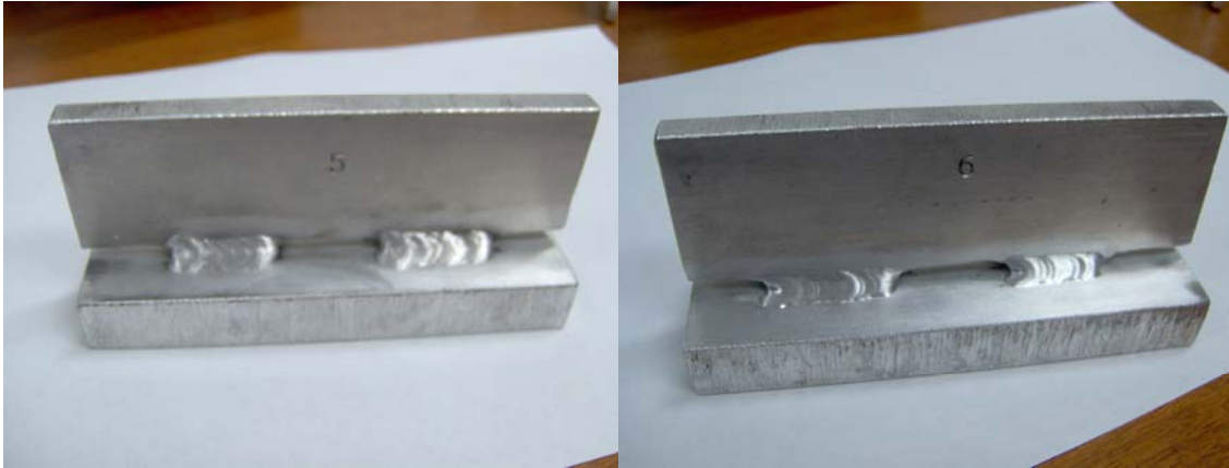
Figure 4 side view of scalloped T-weld Weld 5 MIG, He-Ar mix ,cold sample Weld 6 TIG, He-Ar mix, sample pre-heated by MIG
