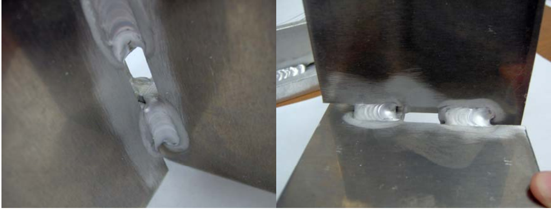
Figure 7 view of cross welds and crevasses. Weld 11 TIG, Ar, cold sample
