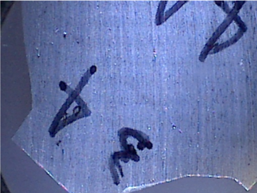
Weld 3&4 slice 4a etched
