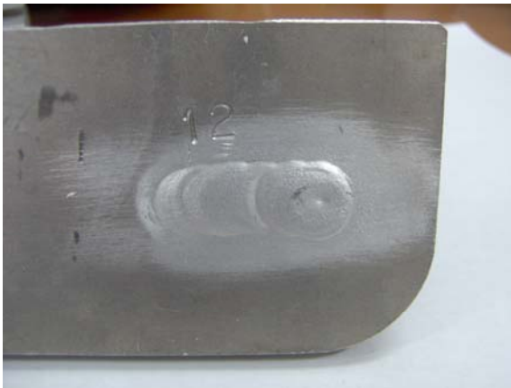
Figure 6, Plug T-welds Weld 12 TIG, He-Ar mix, sample pre-heated by MIG Weld 13 MIG, He-Ar mix, cold sample
