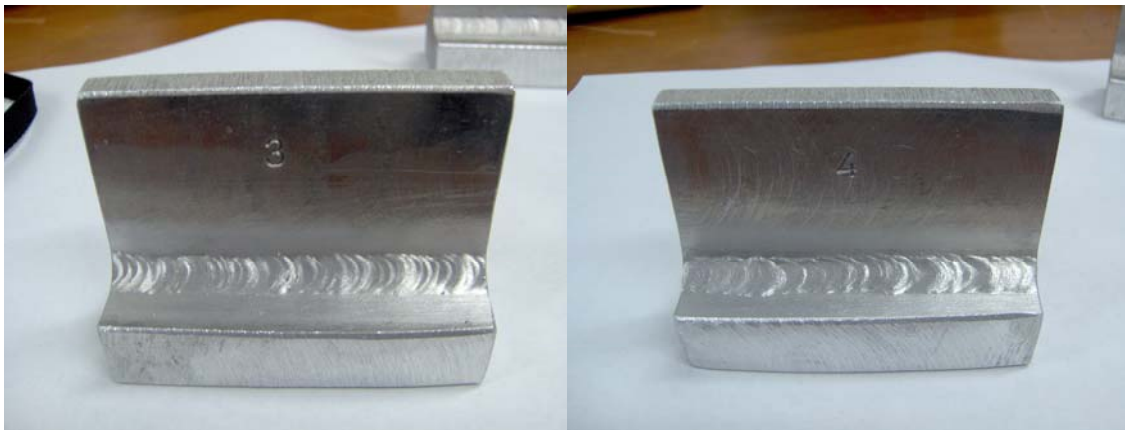
Figure 2: Welds of sample 2 Weld 3 TIG, Ar, sample pre-heated by MIG Weld 4 MIG, He-Ar mix, cold sample
