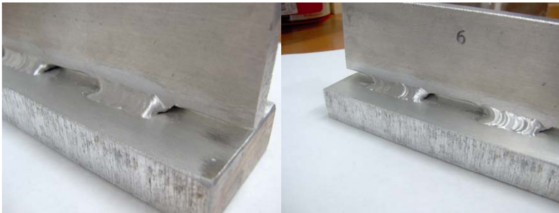
Figure 5 View of the ends of welds 5 and 6 Weld 5 MIG, He-Ar mix ,cold sample Weld 6 TIG, He-Ar mix, sample pre-heated by MIG
