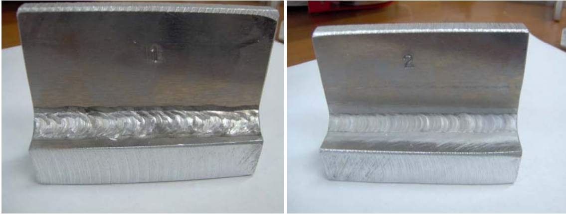
Figure 1: welds of sample 1. Weld 1 MIG, He25%-Ar75% mix ,cold sample Weld 2 TIG, He-Ar mix, sample pre-heated by MIG
