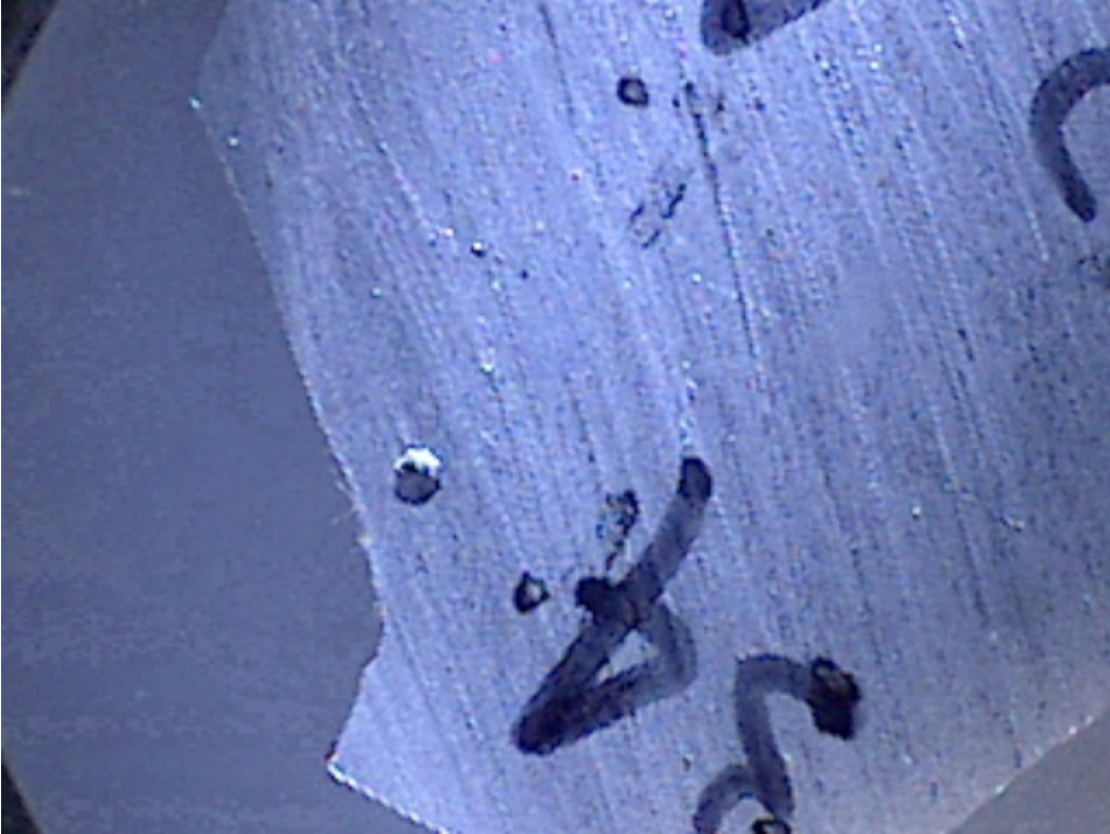
Weld 3&4 slice 3a side 4 etched
