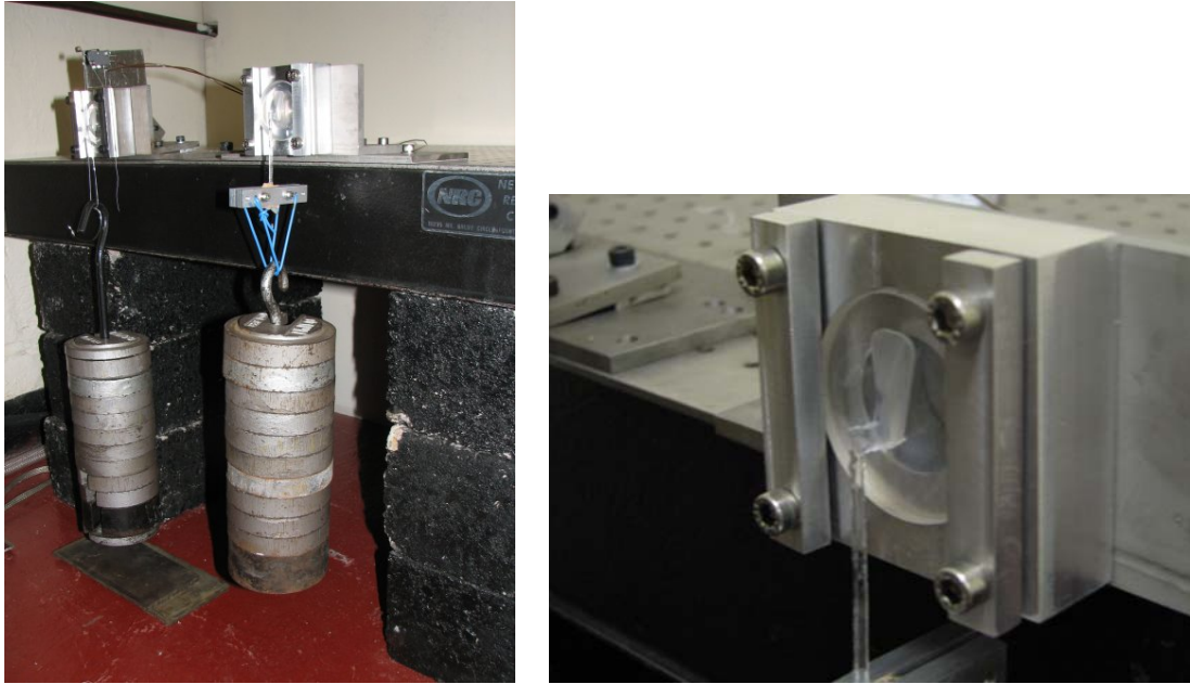
Figure 2a & 2b 12.5 kg suspended from laser welded rod on bonded Preliminary Test Ear SN0003 (20 th Jan 2006)- right hand side of photo
