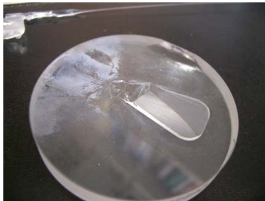
Figure 4 Failure location in ear showing torn silica – bond does not appear to have been compromised.
