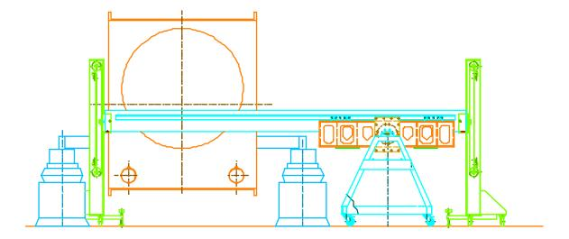
Note that, although bench loading with its optical payload and ballast, as well as balancing, can be done inside the HAM chamber, this operation is much more easily performed externally, while the bench is still sitting on its cart.
