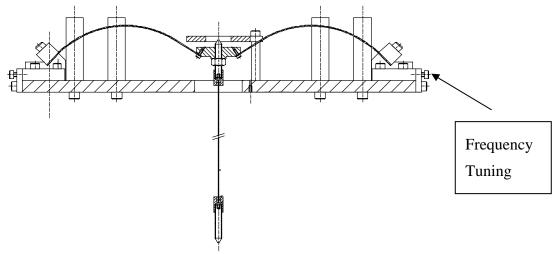
The resonant frequency tuning of a filter is a robust setting, much less sensitive to thermal and mechanical changes than the vertical working point. Requiring that the vertical working point does
