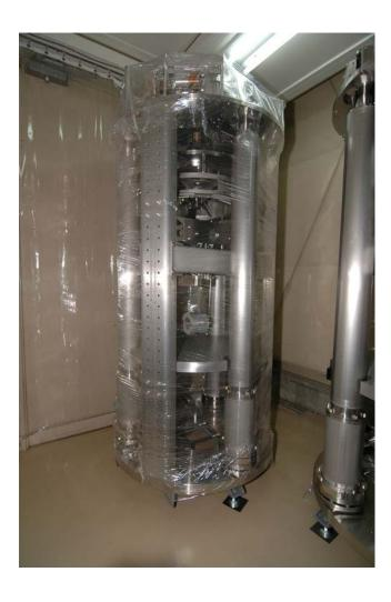
View of a TAMA SAS unit preassembles, tuned and packaged in a NAO clean room, ready for transportation and installation in the main TAMA experimental hall
