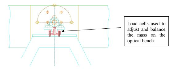
After this the entire optical bench can slide in place horizontally and only minimal adjustments of ballasts will be necessary, to compensate optics re-positionings or last minute replacements. The optical bench sits on a kinematic mount and will not require bolting. Only hooking of the parasitic tuning springs and connection of electrical cablings will be necessary.
