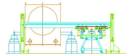
The unit is pushed into the HAM chamber, lowered 450 mm to fit over and be bolted to the cross tubes.
