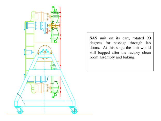
When in front of the HAM chamber the SAS unit is rotated into its horizontal position.
