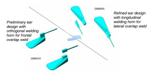
*Figure 3 Refinement of ear from design with orthogonal welding horn (D060018) to longitudinal welding horn (D060055). Ribbon modifications are discussed in Section 4.6.*
