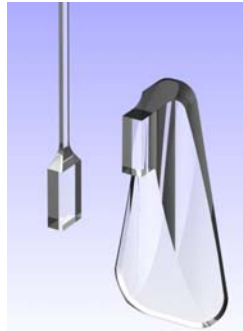
Figure 4 Sketch of preliminary ear for test mass showing triangular footprint to minimize bond peeling effects. The horn has been designed to accommodate lap-welding of the thickened ribbon head. The design details of this horn have yet to be optimized. The ear shown has since been modified to increase the radius at the horn to minimize stress concentration in this region. Note that similar ears (orientated at 180°) will be used on the penultimate mass with no technical noise restriction on bond area.
