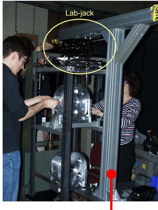
NOTE: Construction of a 'gallows' structure (incorporating a lab-jack to interface with/lift the UI mass) adjacent to the 3&1 Assembly setup
