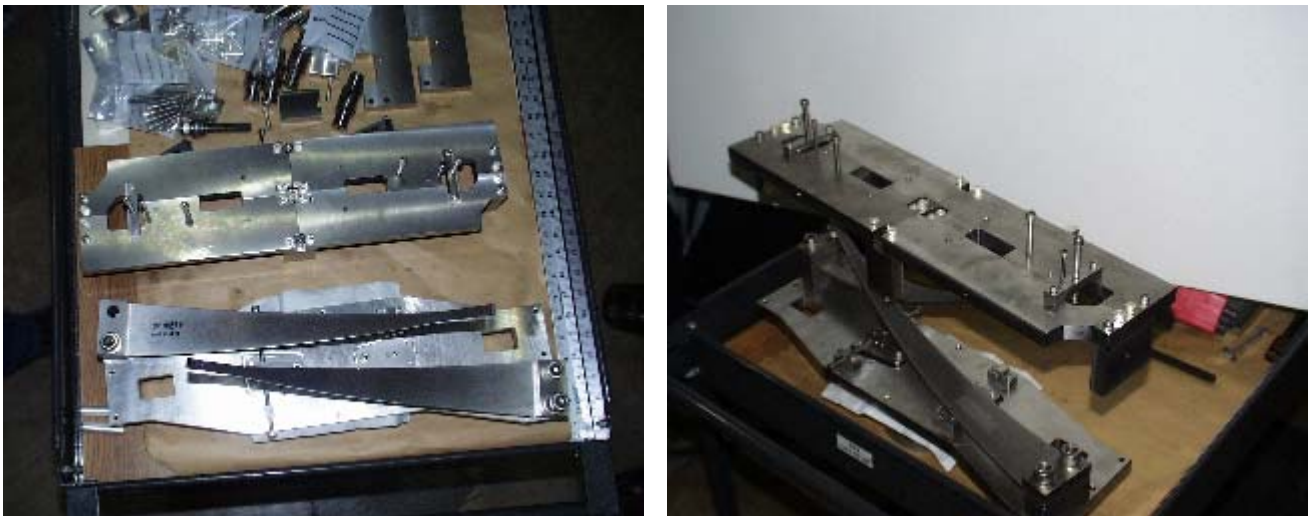
FIGURE 1: C-Ptype ETM Top Mass Build October 2004 – Left View: Top half and bottom half with blades; Right View: Top half above bottom half prior to blades being flattened.
