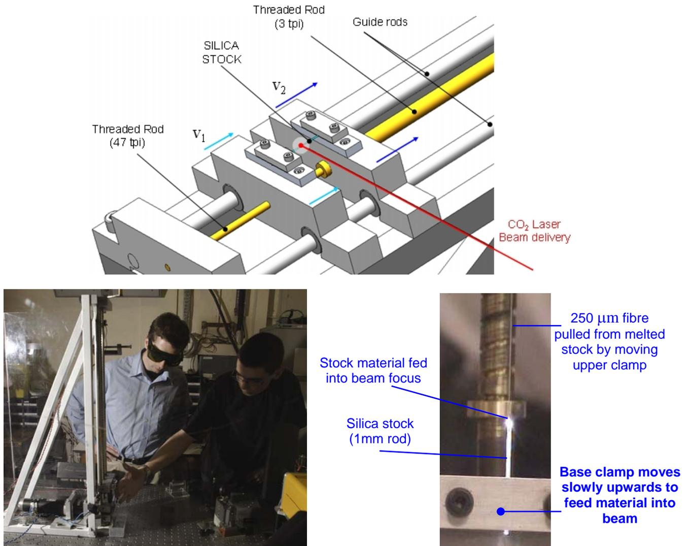
Figure 3 (a) CAD representation of the pre-prototype set-up; fixed ratio of ‘feed’ ( $v_1$ ) to ‘pull’ ( $v_2$ ) = 1:16. (b) Pre-prototype set-up in the lab in Glasgow (c) Photograph of the fabrication of a 250  $\mu\text{m}$  fibre - 1 mm silica rod fed into the CO2 laser beam by the slowly moving base clamp as the upper moving clamp draws the fibre.
