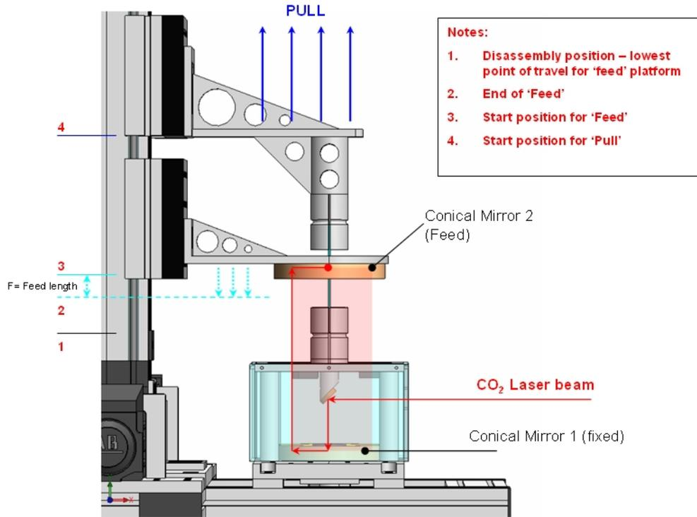
Figure 8 *Feed & pull set-up for production of cylindrical fibres on prototype machine (manufacture and assembly of the beam shaping design in progress)*
