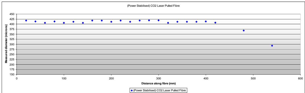
Figure 9 *Dimensional assessment of an early CO<sub>2</sub> laser pulled fibre, pulled on the prototype pulling machine with laser power stabilization.*
