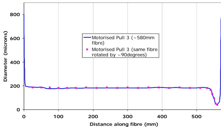
Figure 4 Graph of dimensional characterisation of a 580 mm long fibre, pulled on the pre-prototype pulling machine
