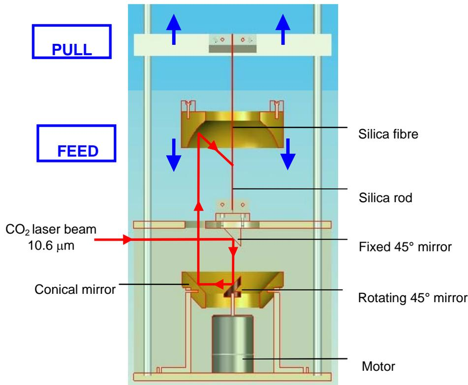
*Figure 2* ‘Feed & Pull’ technique.
