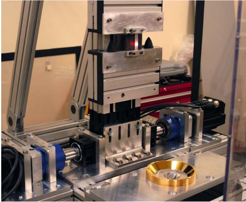
*Figure 7* Ribbon fabrication on prototype machine: silica slide being heated by the dithering of CO<sub>2</sub> laser beam across its width. Gold coated conical mirror used to produce cylindrical fibres also shown.
