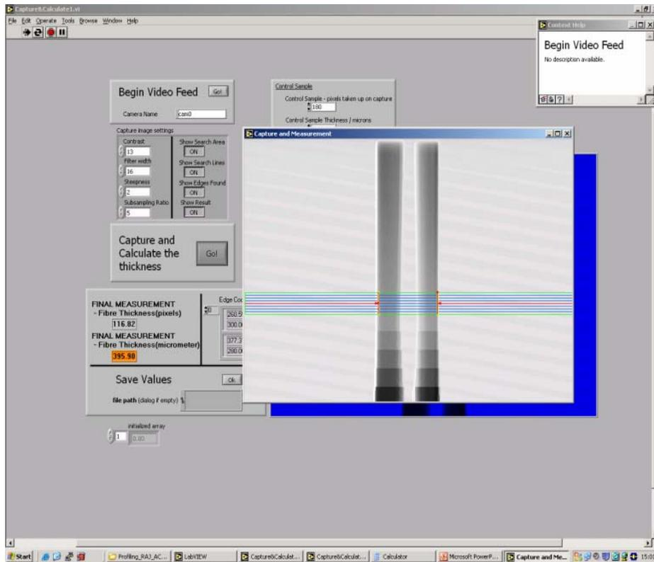
Figure 10 Typical screen capture using a CO<sub>2</sub> laser pulled fibre of ~400 $\mu$ m
