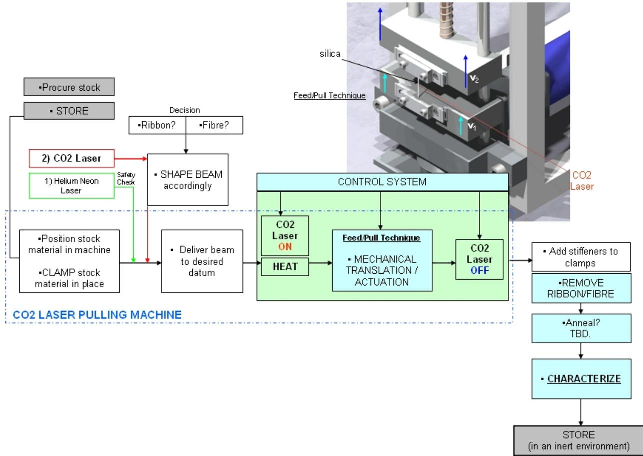
Figure 1 Overview of ribbon/fibre fabrication
