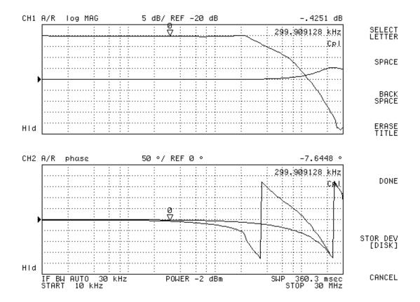
Transfer function of channel 2. (This board had a 10MHz butterworth filter.) Flat(er) trace is measured against a BNC barrel.
