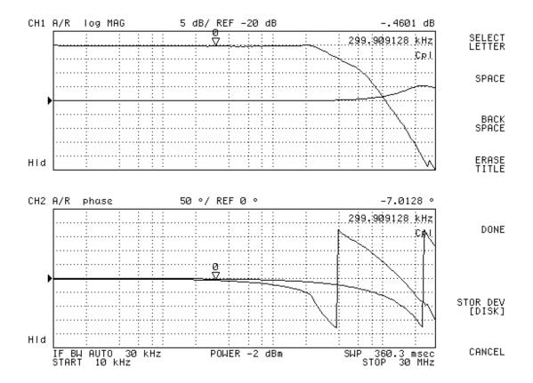
Transfer function of channel 1. (This board had a 10MHz butterworth filter.) Flat(er) trace is measured against a BNC barrel.
