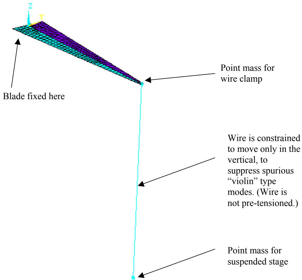
For the time being I left the wire diameter and length fixed.
