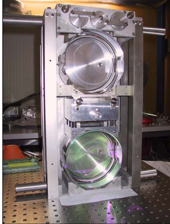
Picture (1 and 2): Picture 1 on the LHS shows one of the main suspensions in GEO 600. Suspended coils can be seen in the aluminum mass in the top left hand side of the picture. Picture 2 on the RHS shows two fused-silica masses in a GEO 600 style catcher / fixture prior to installation into one of tanks.
