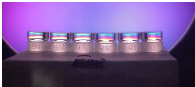
Substrates 50; 44; 49 baked at 120°C for 24 hrs. Substrates 45; 48; 47 baked at 60°C for 24 hrs.
