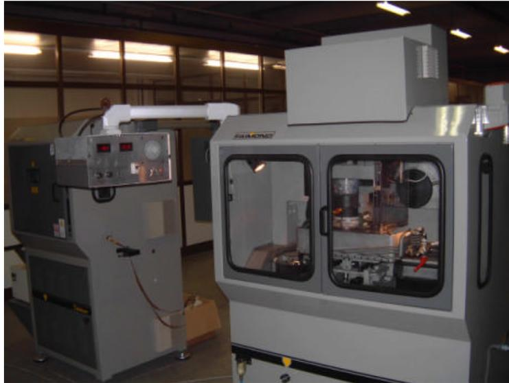
Fig.5 Front view of the 5-axis ultrasonic cutting machine prototype. On the left side is visible the ultrasonic generator, with power and frequency controls. On the right, not visible in the picture, are mounted the PC for the axis control and the 9 inches CRT camera.
