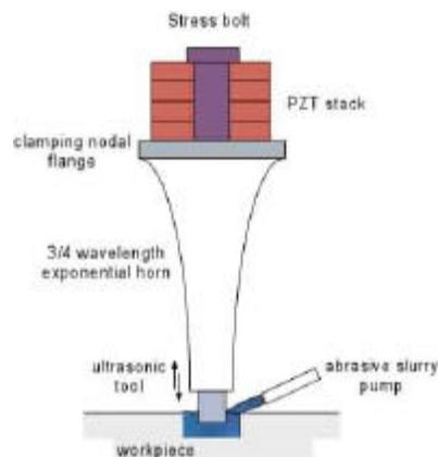
Fig.2 Ultrasonic machine tool schematic
