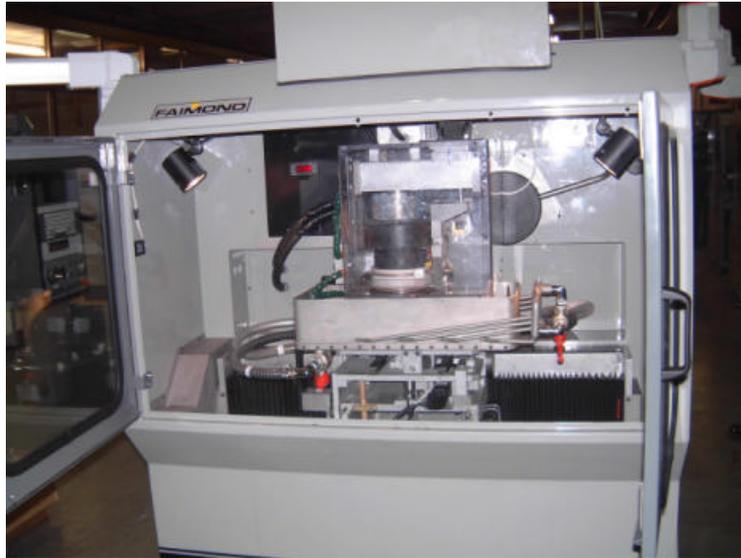
Fig.6 Internal view of the machine. A polycarbonate transparent box (for high voltage safety) hosts the rotating ultrasonic head with the centering slides and the piezoelectric transducer cooling system. The working table is surrounded by the anti-splash container and by the secondary high-flow slurry feeding. Below the table (the protection carter has been removed) is visible the load control system.
