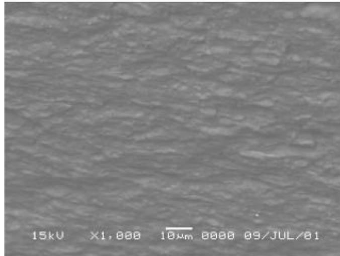
Fig.3 SEM micrograph of a single crystal sapphire surface machined in our laboratory with boron carbide 220 mesh. Irregularities of 1-5  $\mu\text{m}$  can be observed.
