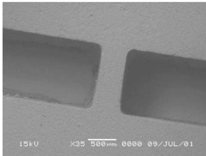
Fig.4 SEM micrograph of a  $400 \mu\text{m}$  thick flex-joint machined from a 3-mm thick sapphire single crystal wafer.
