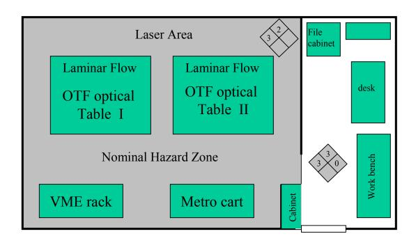
Figure 1: The OTF Laboratory Floor Plan
