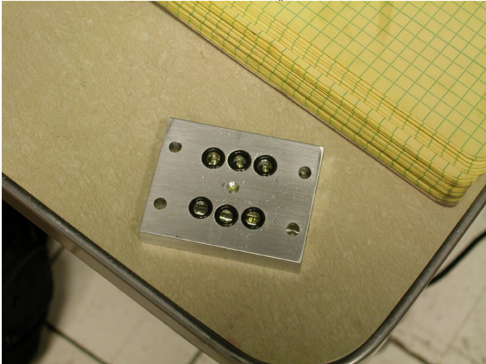
This is a dummy valve, which is placed on the flowbench in place of a Parker valve. Its purpose is to establish a zero resistance baseline before the valves are tested.
