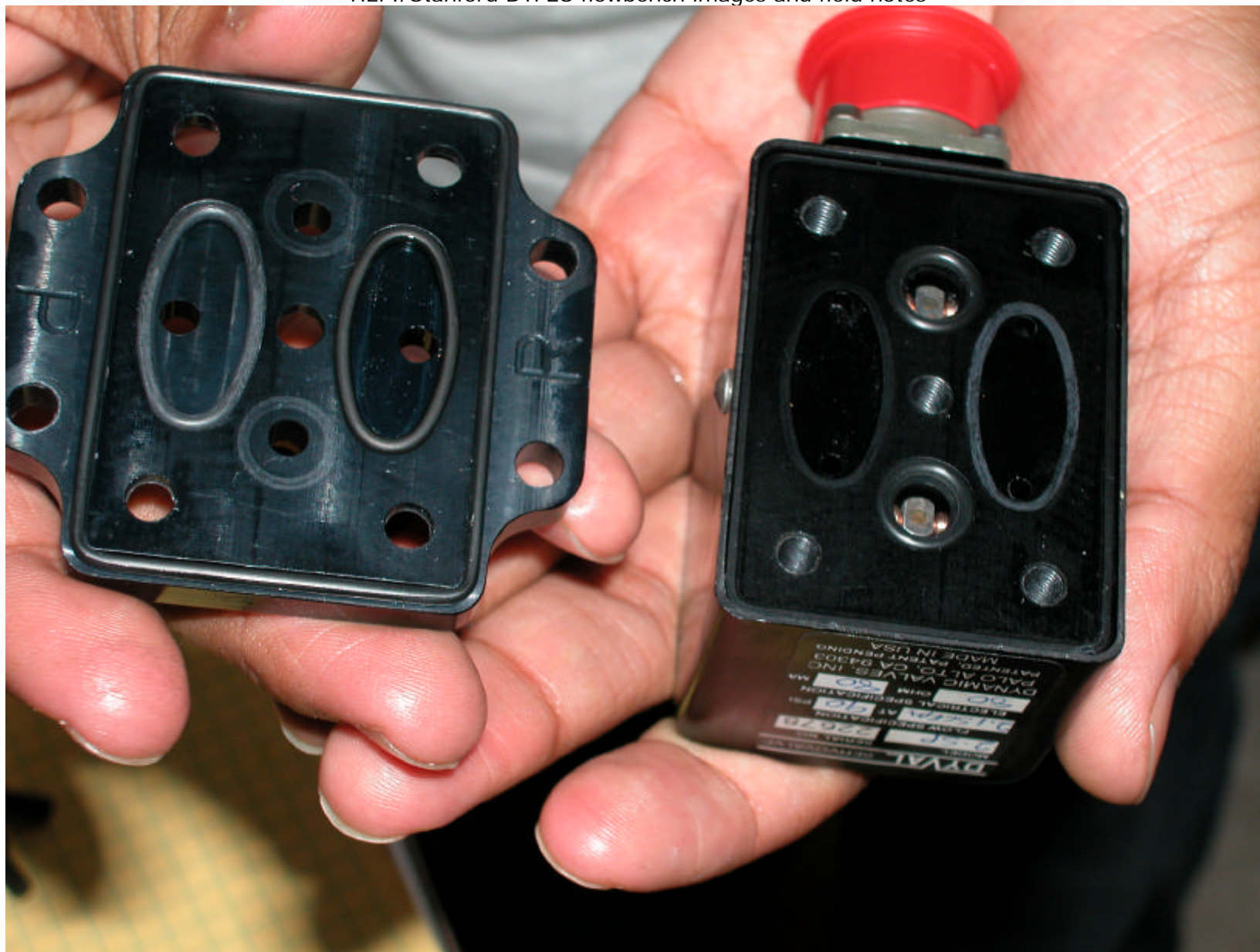
Parker DYP2S with baseplate removed. 4 nozzles can be seen on right. Two nozzles are combined through the elliptical port seen on left
