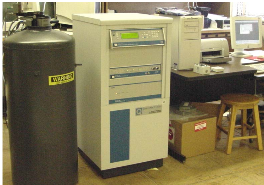
Picture 19: PPMS cryostat used for thermal conductivity measurements
