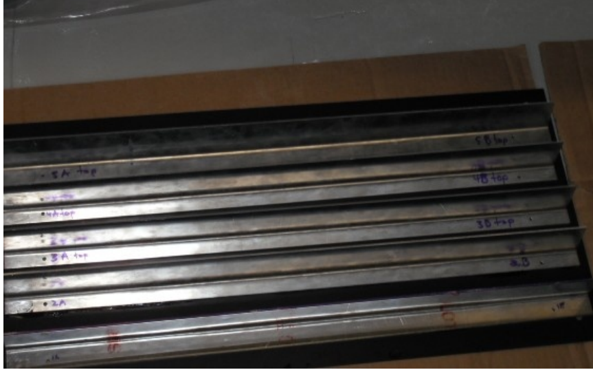
Figure 1: The holes were marked on both the L's and the black aluminum so when more drilling and riveting occurred the holes would be in the right places.
