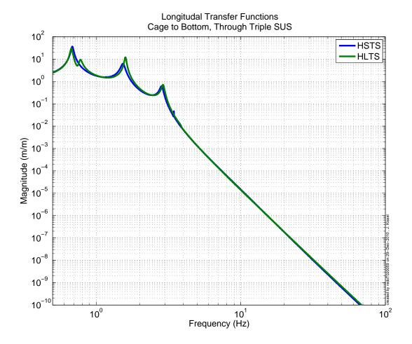
Figure 2: Transmission of HAM ISI input displacement noise through the HSTS and HLTS their respective the bottom masses,  $T_{x \to x}^{p \to B}$ . Models are computed using T080311 and T080310.
