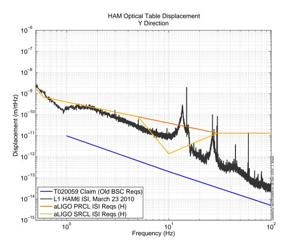
Figure 1: Comparison between requirements and measurements of the HAM isolation platform motion,  $x_p(f)$ . In blue, that which is defined by T020059-v1 (taken to be the same as the BSC platform, originally defined in E990303); in drak gray, the eLIGO HAM6 ISI performance (in the Y direction); in orange and gold, the requirements defined for the PRCL and SRCL HAM ISI in Advanced LIGO from T1000216, respectively.
