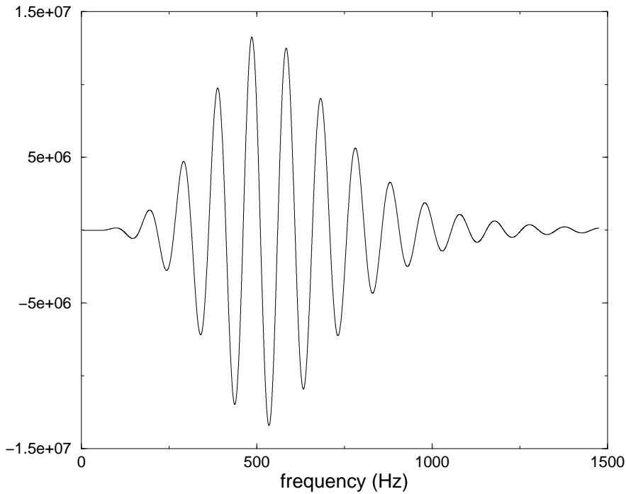
Figure 1: Optimal filter for cross-correlations between LIGO Livingston and LIGO Hanford, assuming an unwhitened noise power spectral density proportional to  $\left(\frac{f}{800\text{Hz}}\right)^{-4} + 3 + 2\left(\frac{f}{800\text{Hz}}\right)^2$ , which is a reasonable “eyeball fit” to the shape of the E2 sensitivity curve available from [3].
