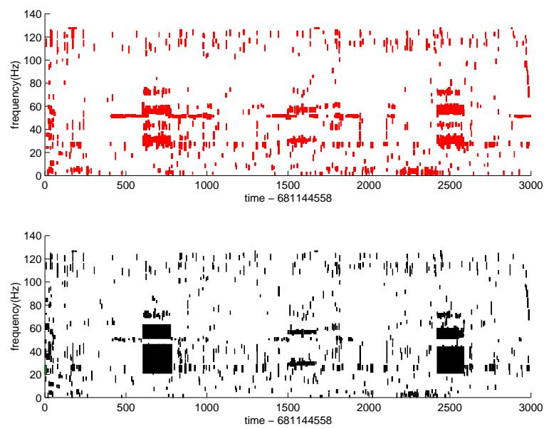
Figure 2: Comparison of output from the LDAS DSO tfclusters (green) and the DMT monitor TID (red).
