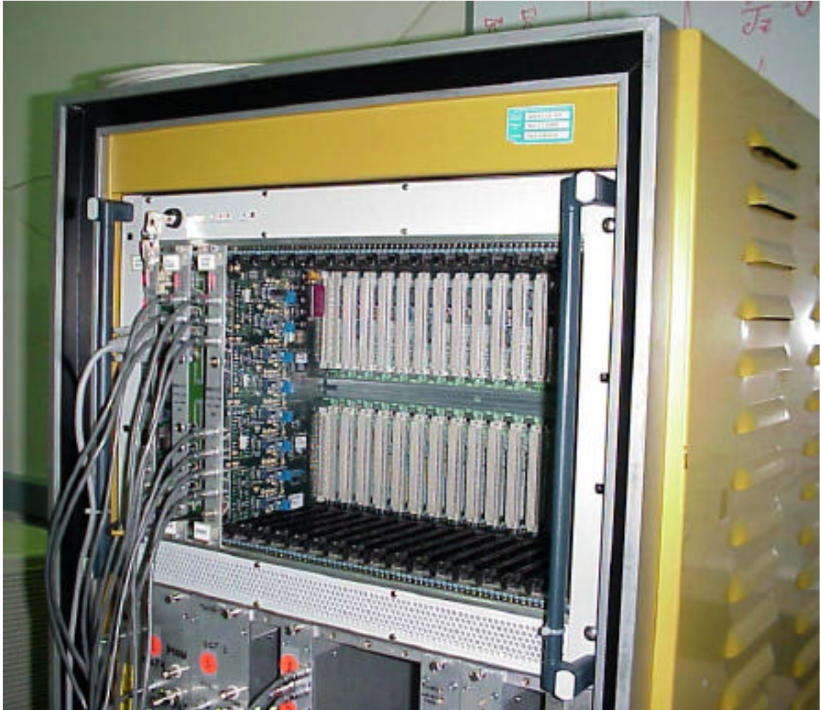
Figure 5: Photograph of the Virgo and TAMA digital control electronics. The three modules in the VME crate are the DSP, the ADC and the DAC cards generating the diagonalization matrices, the frequency filters and running an entire SAS tower local controls. A group of modules identical to these three will manage the interferometer global controls.
