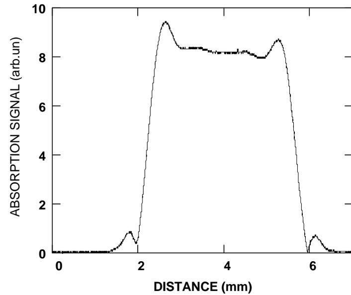
**Example: 3 mm-thick neutral filter, 15%-absorbing**
