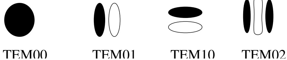
Fig 1. Transverse profiles of TEM modes
