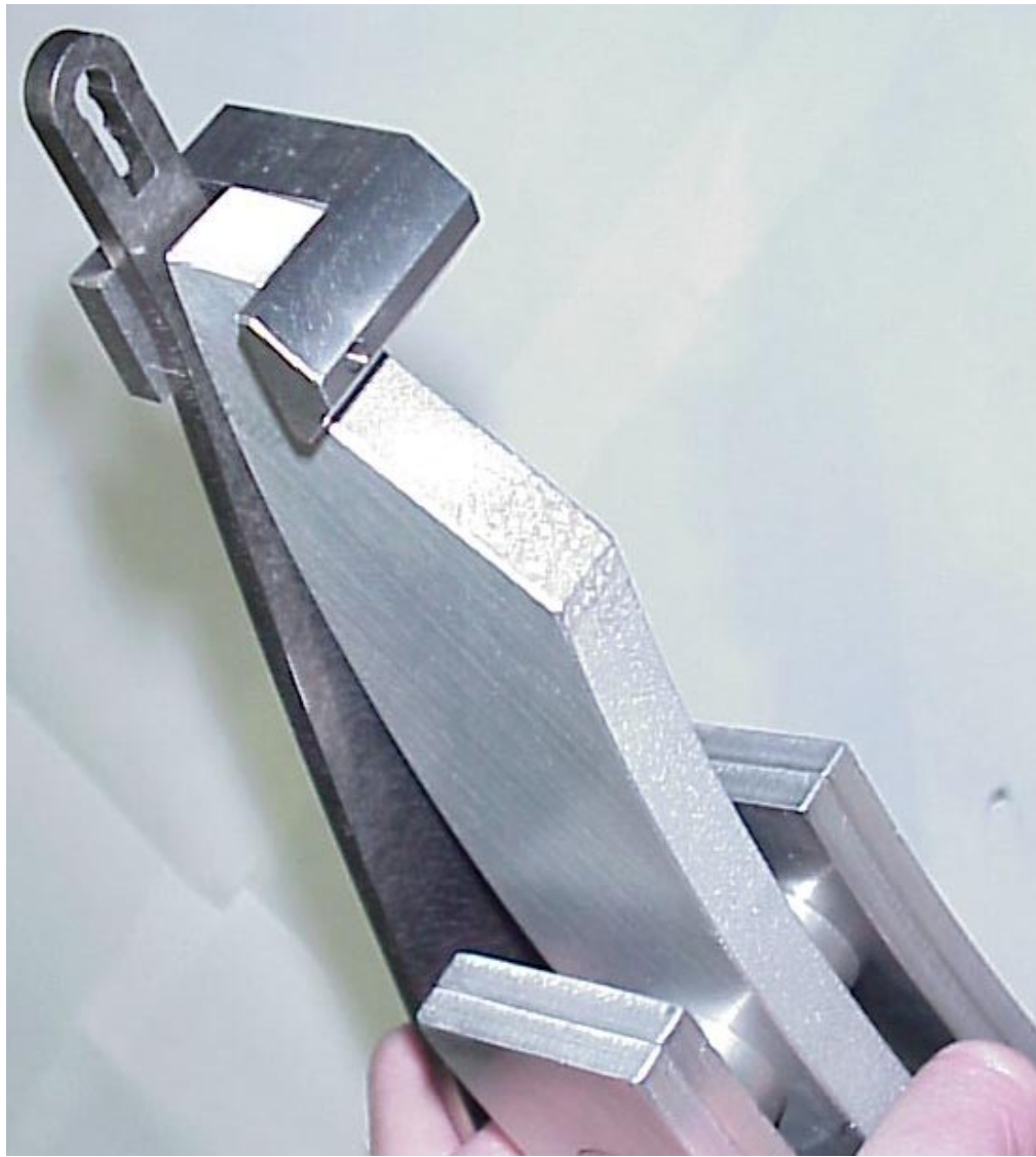
Figure 4.9: Assembly time, strap to keep the blade bent
