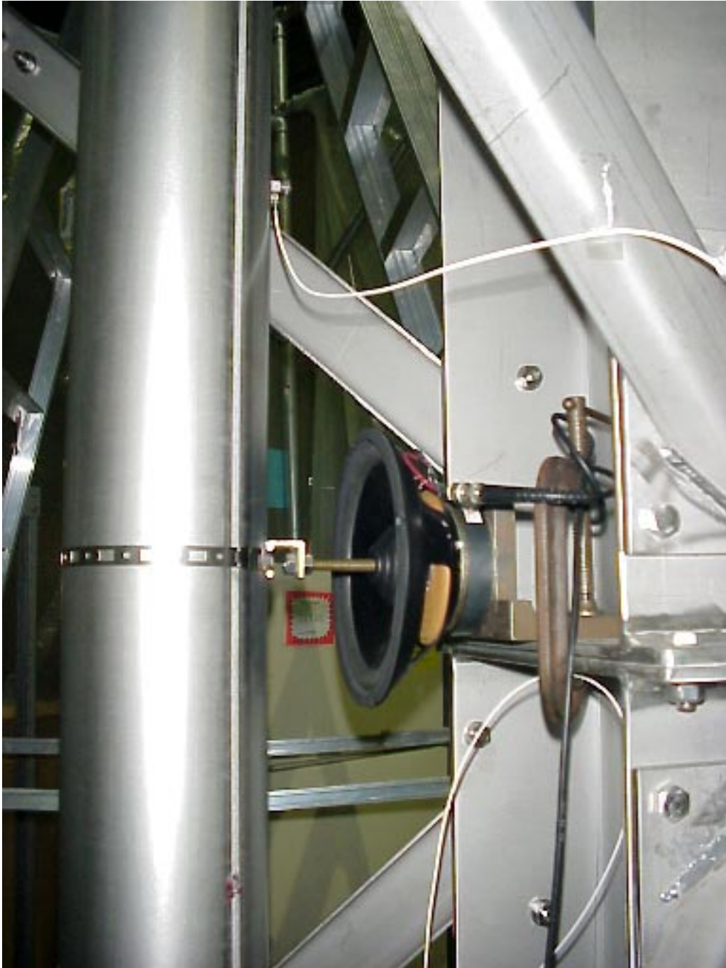
Figure 2.4: Loud speaker used to excite the leg, and accelerometer.
