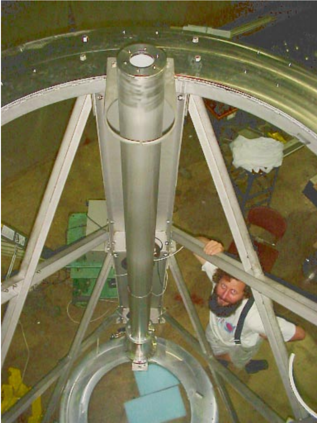
Figure 2.2: Inverted pendulum leg surrounded by the safety structure.
