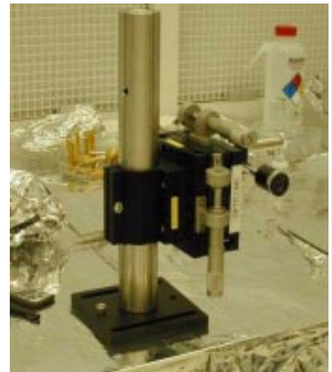
Traveling microscope, mount, and vernier adjustments
