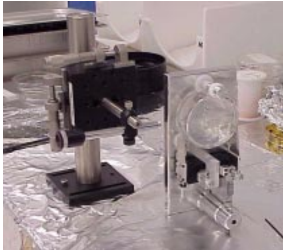
Gluing fixture/optic assembly and traveling microscope.
