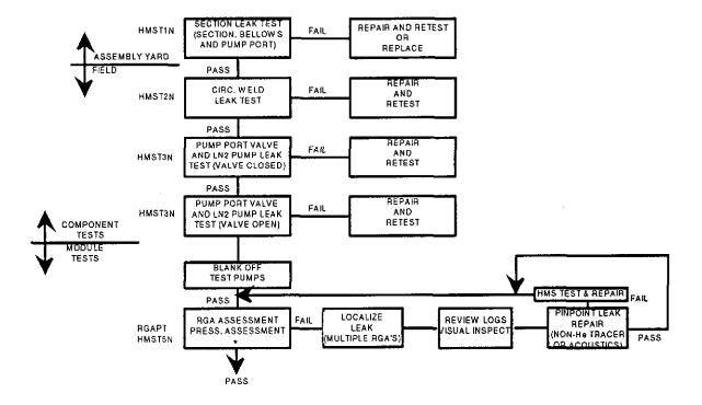
\* Acceptance criteria is: Two times the smallest detectable leak which must be smaller than 1E-5 atm. cc/sec. but no smaller than 2E-8 atm. cc/sec.
