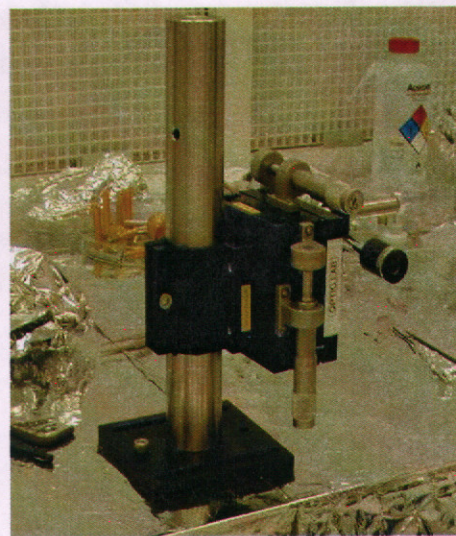
Traveling microscope, mount, and vernier adjustments
