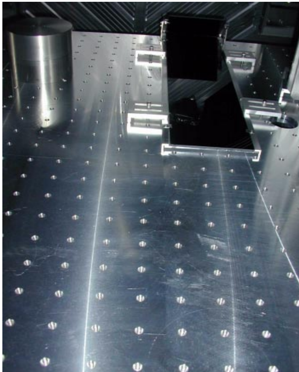
HAM 9 COS RM Ghost Beam Beam Dump. North is at the top.
