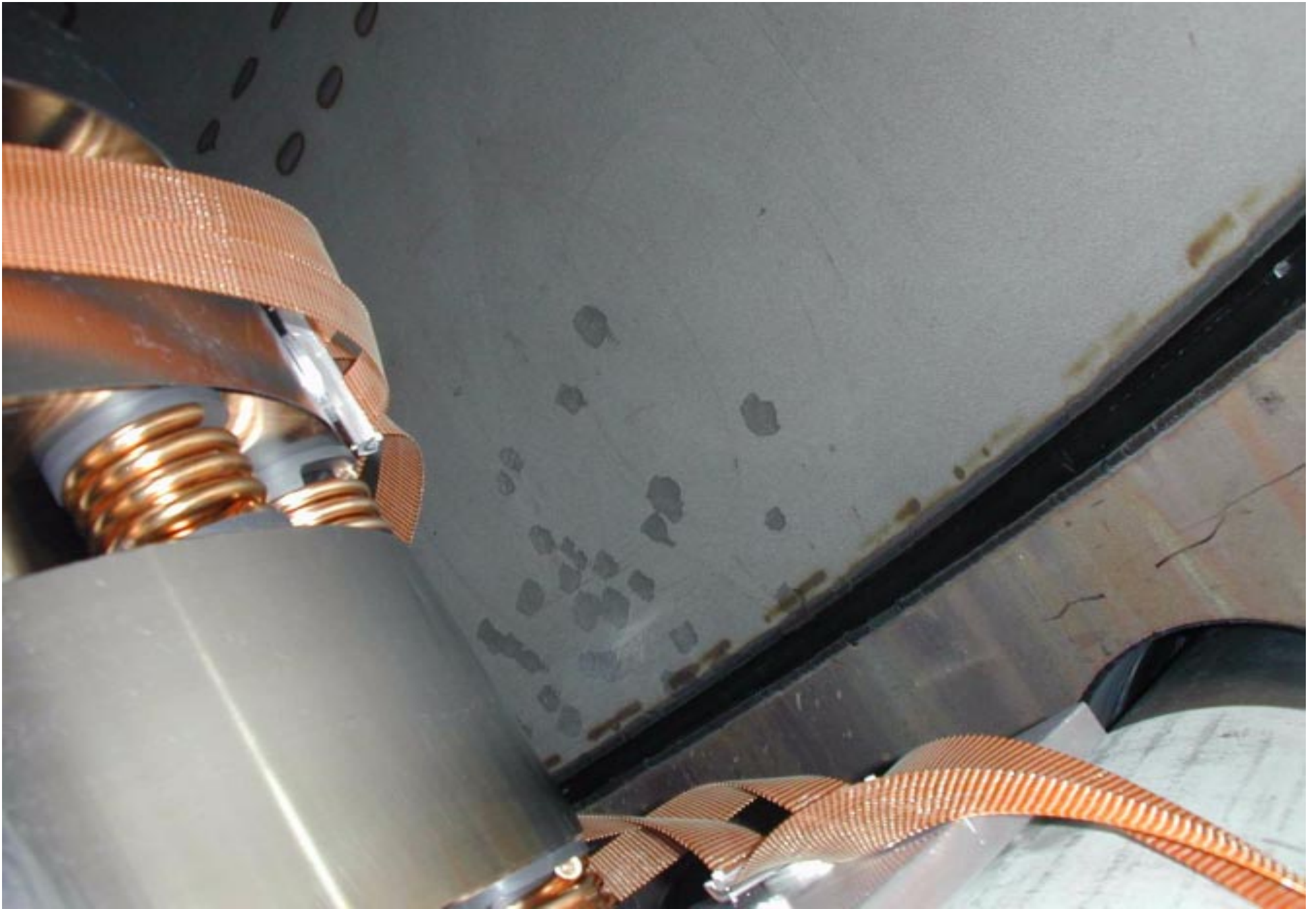
BSC 10 SE Seismic Stack and support tube with ribbon cables.
