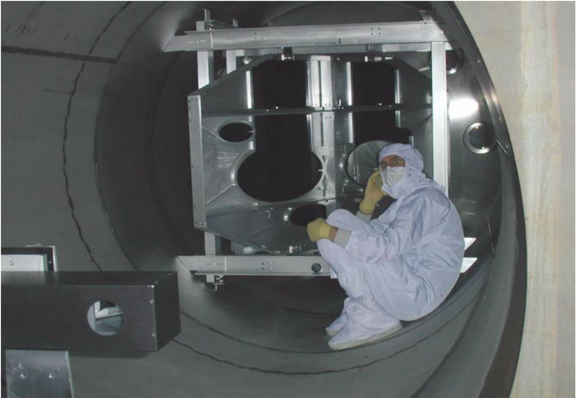
BSC 10 Arm Cavity Baffle as viewed from the BSC10 chamber looking towards the vertex. 4k beam hole is behind Rick Savage on the right. PLX alignment equipment is in the foreground.
