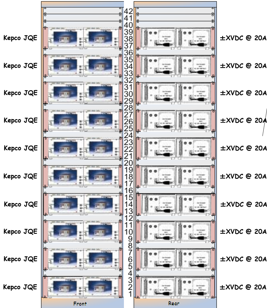
DC Power Rack
