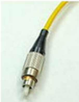
FC Ferrule Connector or Fiber Channel
