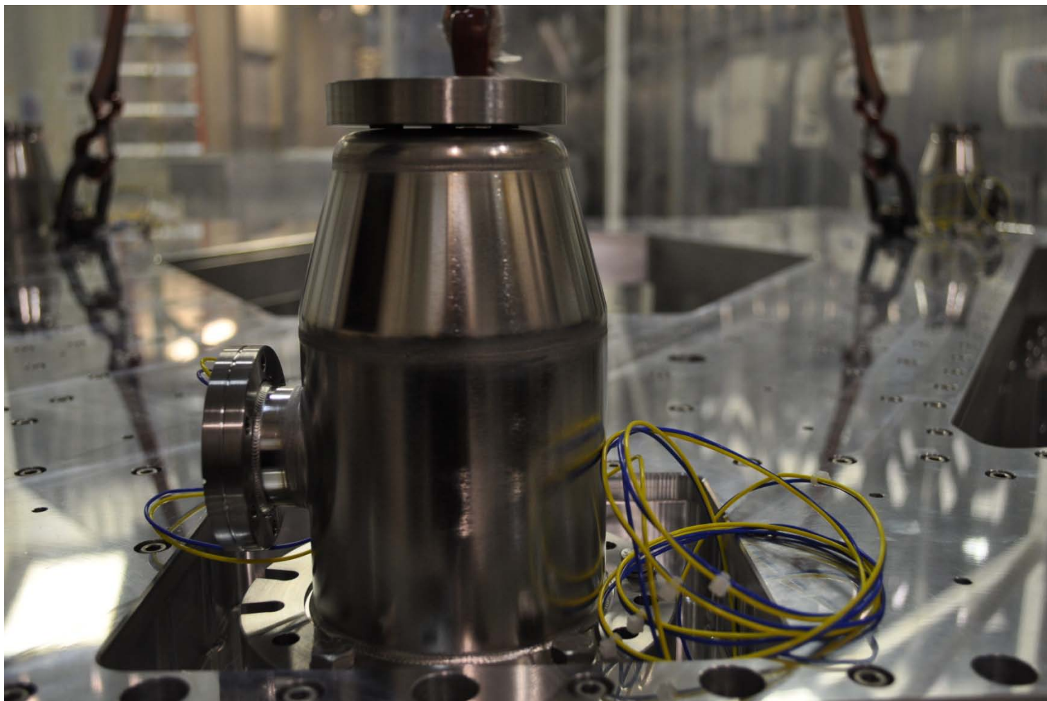
1 Lb Mass Damper on the top of the L4Cs
