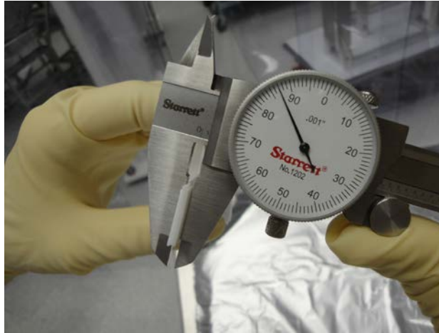
Figure - Stack of Teflon shims being measured for gap check of actuators.
