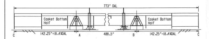
Assume that the end plate of the casket clears the tube by  $\frac{1}{6}$ " when the casket is in place. What is the difference in elevation of points A and B to close that gap to zero at point C? delta h = .125(488.5/142.25) = .43"
