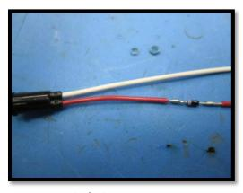
d. Slide a 1 ½ piece of 1/8 "shrink wrap over diode and exposed conductor and apply heat.
