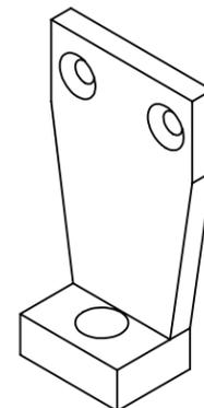
DRILL AND TAP FOR 1/2-13 UNC N60 HELICOIL INSERT #1185-8EN500 THRU
