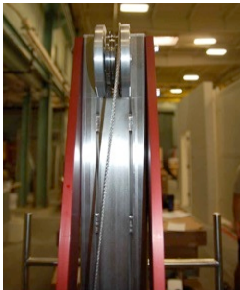
Figure 4: Wire laying to the right of its track
