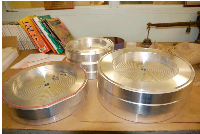
Figure 2: TM vacuum plate on left, FM's on the right and R's in the back.
