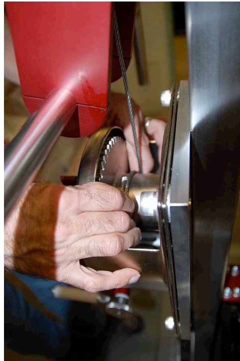
Figure 6: Fixing the wire, it should wind onto the spindle from left to right, viewed this way.
