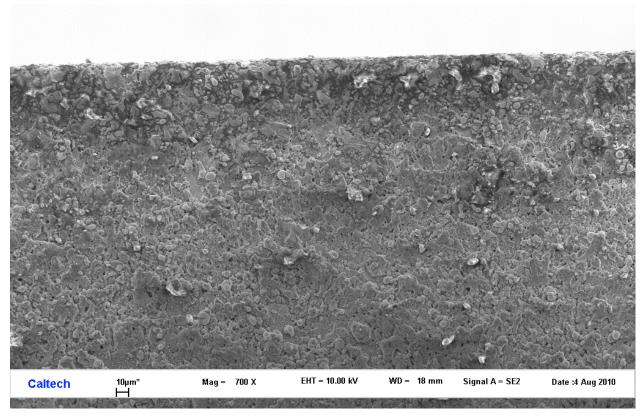
The image above was taken of the unpolished, uncoated knife-edge and has protrusions along the blade.
