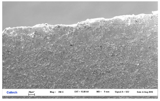
The image above was taken of the DLC PVD coated knife-edge. The DLC PVD structure given by LAFER, the manufacturer, is: Cr flash + glassy WC (2.5 um) + 0.5 um of Carbon CVD.
