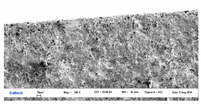
The image above was taken of a polished, uncoated knife-edge and does not contain protrusions along the blade as seen previously on the unpolished knife-edge.
