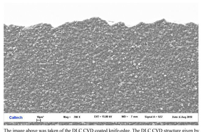
The image above was taken of the DLC CVD coated knife-edge. The DLC CVD structure given by LAFER, the manufacturer is: 2.8 um of Carbon CVD. The coating appears to have conformed perfectly to the surface.
