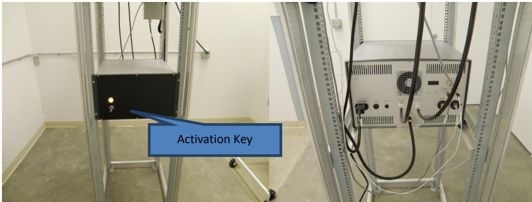
Figure 7: The pump laser diode (PLD) box front and rear view.
