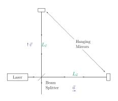
Laser interferometer measures strain h, given by
