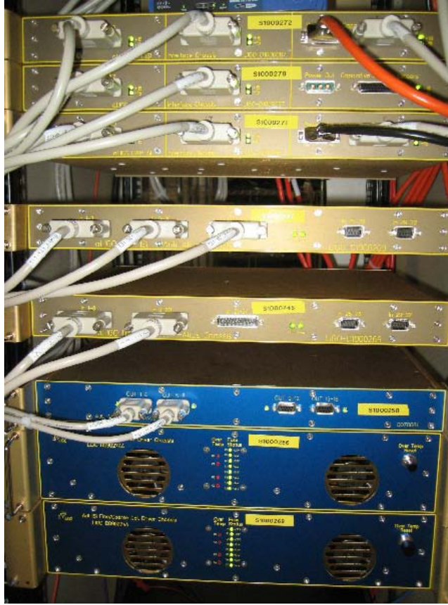
Figure - From top to bottom – Interface chassis – Anti-aliasing filters Anti-image chassis – Coil Driver
