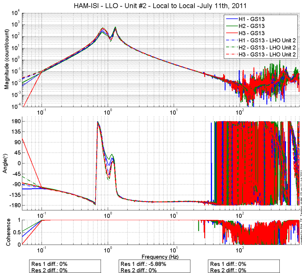
Figure - Local to local measurements comparison with LHO HAM Unit 2 – Horizontal GS-13
