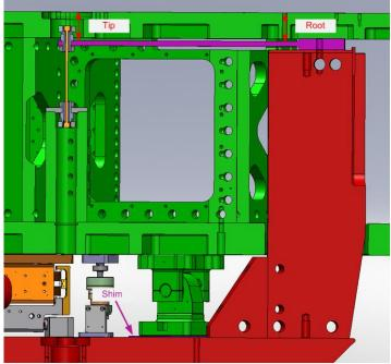
figure – Blade spring profile measurement points
