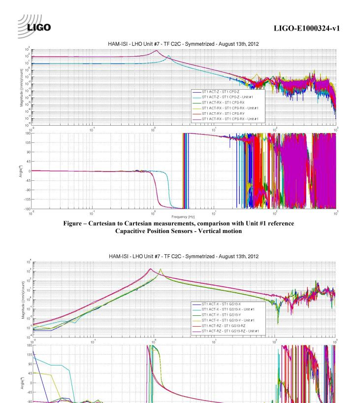
Figure – Cartesian to Cartesian measurements, comparison with Unit #1 reference – Inertial Sensors Horizontal motion
