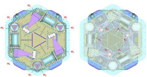
Figure – Wall Masses (W) and Keel masses (K) location. South of picture = corner 1
