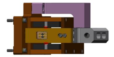
Figure - Showing gaps that need to be checked on actuators.
