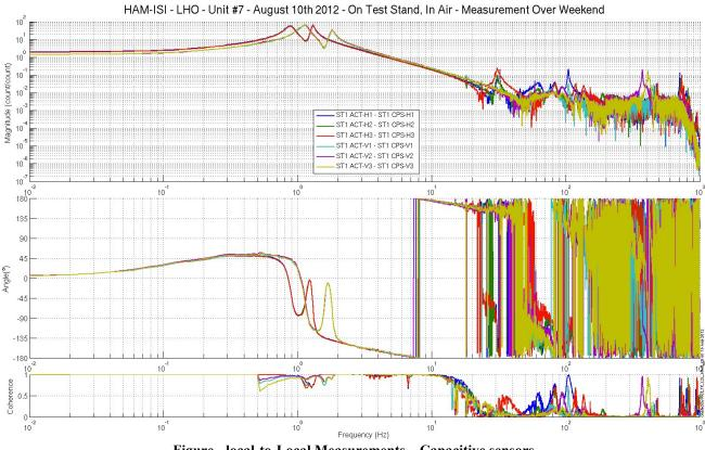
Figure - local-to-Local Measurements - Capacitive sensors
