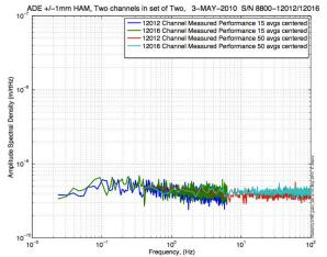
Figure - H2 and V2 sensor noise
