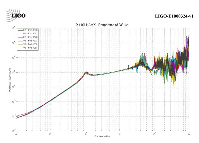
figure - Extracted GS13 responses comparison
