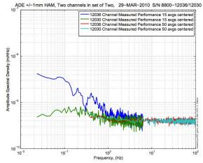
Figure - H3 and V3 sensor noise
