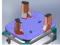
Figure - Showing edges that need checked on support posts and gussets
