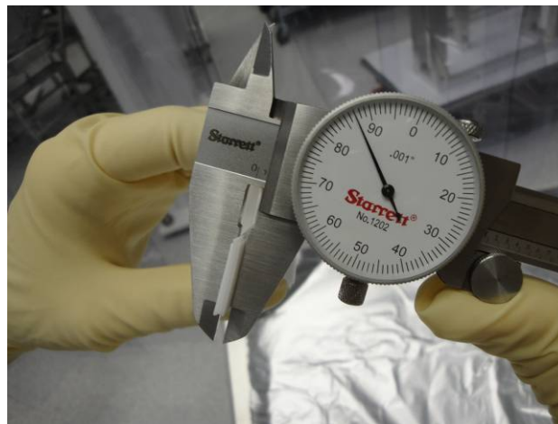
Figure - Stack of Teflon shims being measured
